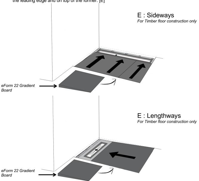
14. Unfold, & overlap flexible membrane from the chassis, so it can be fixed onto the upper surfaces of the eForm 22 gradient boards, or any other horizontal surfaces of the floor, and/or the vertical surfaces of the wall. Secure using tile adhesive, ensuring the drain chassis is completely sealing into the shower area structure.
